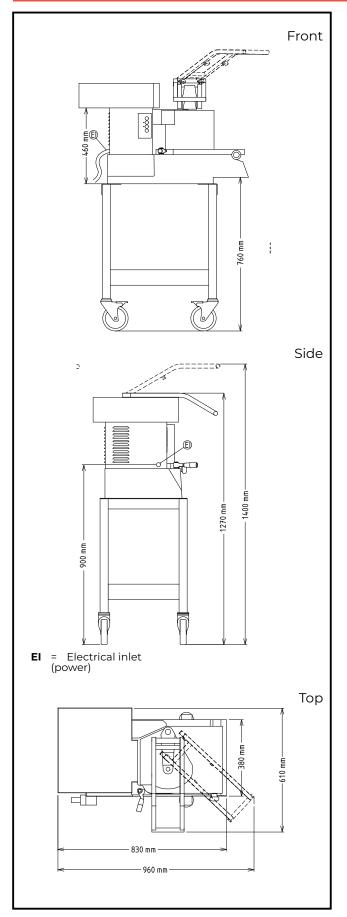
Electric Supply voltage: 380-415 V/3 ph/50 Hz Electrical power, max: 2 kW **Total Watts:** 2 kW Capacity: Performance (up to): 700 kg/Cycle Key Information: External dimensions, Width: 610 mm External dimensions, 830 mm Depth: External dimensions, Height: 1400 mm
